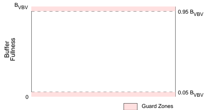
Figure 10.3: Guard zones to safeguard against underflow and overflow of VBV buffer. A bit allocation is computed so that the buffer fullness remains between the guard zones.
