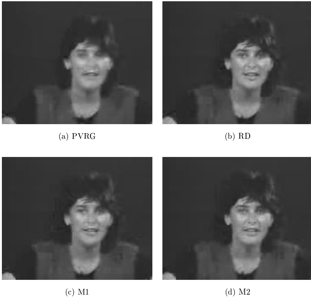
Figure 3.7: Frame 27 of the Miss America sequence as encoded using the PVRG and explicit-minimization motion estimation algorithms. Only the luminance component is shown.
